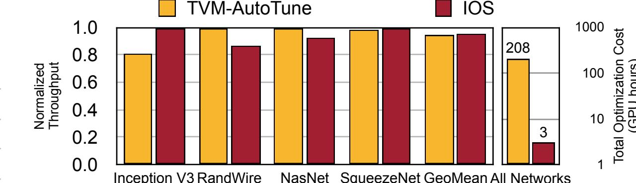
AutoTVM and IOS are **orthogonal** and can be combined to further boost the performance
