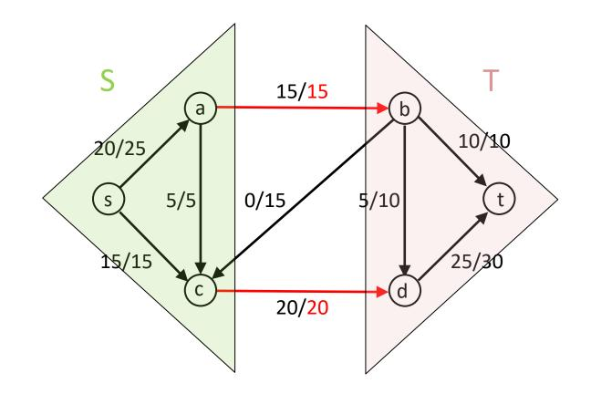
capacity of (S,T) cut = 35 no flow can have value that exceeds this  $\Rightarrow f'''$  is maximum flow
