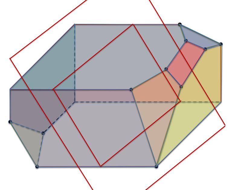
Geometry of LPs with 3 variables. The objective function: set of parallel planes
