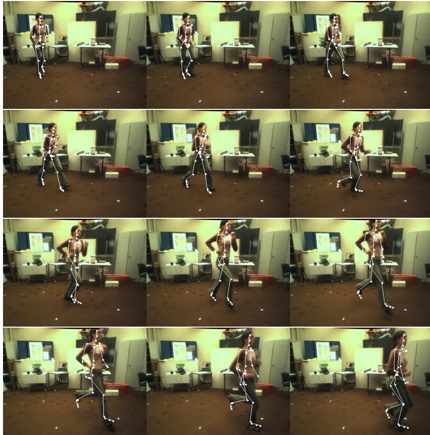
Fig. 11. Tracking the transition between walking and running. In the first four frames the subject is running. The transition occurs in the following three frames and the sequence ends with running. The whole sequence is shown.
