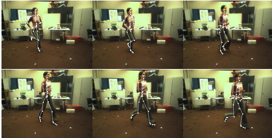
Fig. 9. Tracking a running motion while allowing the style to vary. The legs are now correctly positioned in the whole sequence.
