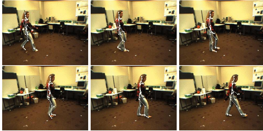
Fig. 5. Using low resolution stereo data to track a woman whose motion was recorded in the database. The recovered skeleton poses are overlaid in white. The legs are correctly positioned.
