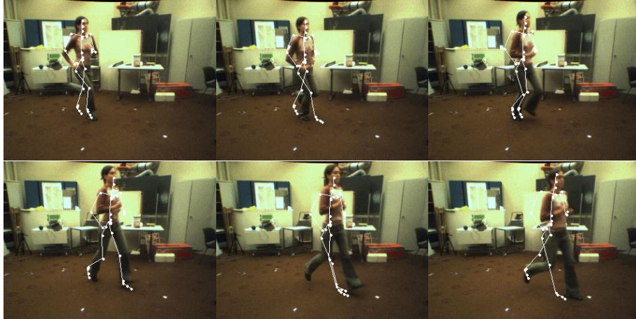
Fig. 3. Tracking without a motion model. Given the low framerate, motion between frames is large enough to provoke erroneous attachments of data points to body parts and, as a consequence, very poor fitting behavior. The whole sequence is shown.
