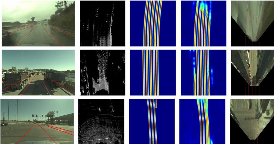
Fig. 6. Failure cases due to rain, occlusions and missing lane markings. From left to right: (1) The detected lane distance transforms are naively thresholded and projected into the camera image using the predicted ground height. Lanes are predicted up to 48m ahead. (2) The LiDAR image. (3) The ground truth lanes. (4) The distance transform output of the model. (5) The camera warped to top-down view using the predicted ground overlaid with the predicted lanes (red).
