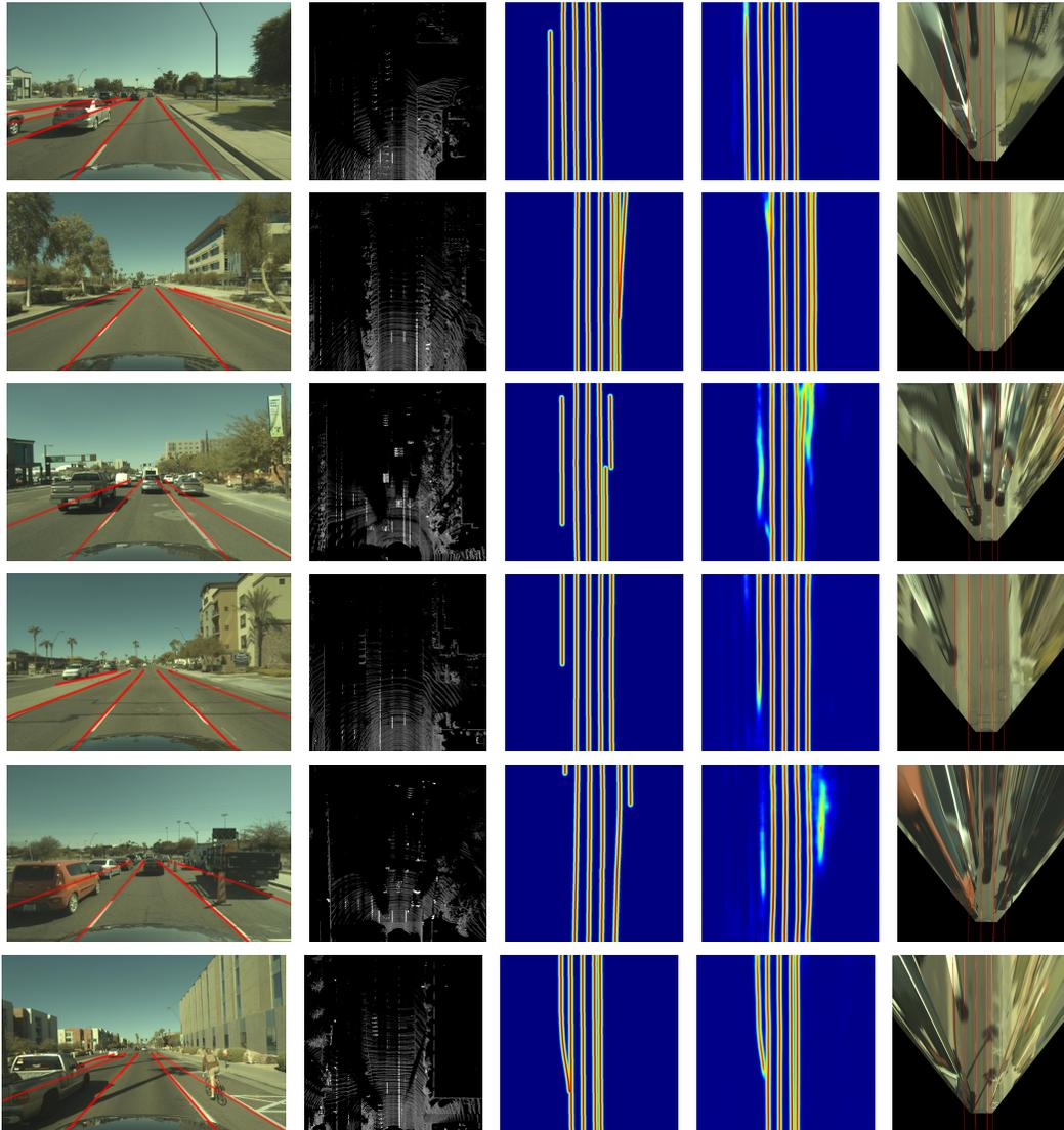
Fig. 5. Output of our method using both LiDAR and camera in urban areas. From left to right: (1) The detected lane distance transforms are naively thresholded and projected into the camera image using the predicted ground height. Lanes are predicted up to 48m ahead. (2) The LiDAR image. (3) The ground truth lanes. (4) The distance transform output of the model. (5) The camera warped to top-down view using the predicted ground overlaid with the predicted lanes (red).
