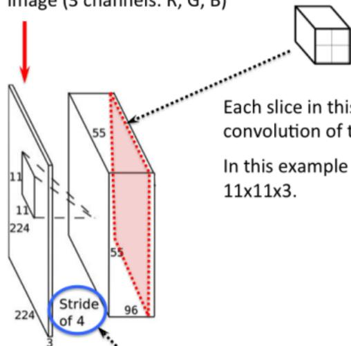
Each slice in this cube is the output of convolution of the image and a filter.
