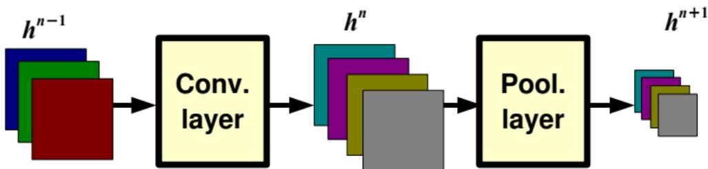
If convolutional filters have size  $K \times K$  and stride 1, and pooling layer has pools of size  $P \times P$ , then each unit in the pooling layer depends upon a patch (at the input of the preceding conv. layer) of size:  $(P+K-1) \times (P+K-1)$
