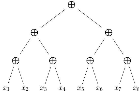
In the above circuit, each XOR gate  $x \oplus y$  can be rewritten as  $(x \vee y) \wedge (\bar{x} \wedge \bar{y})$ .
