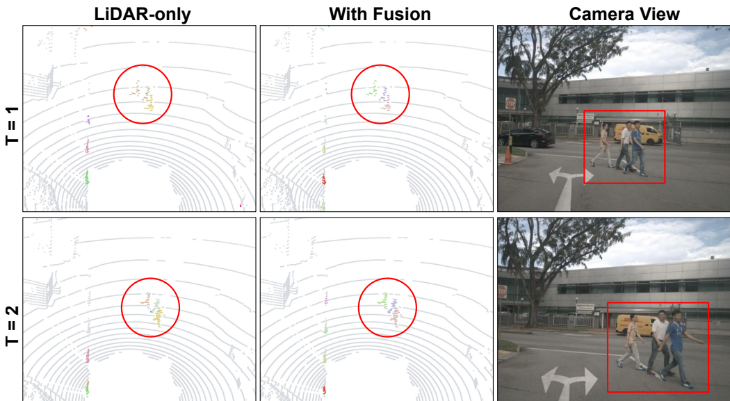
Figure 8: Qualitative comparison of instance segmentation and tracking for LiDAR-only vs. fusion model on sequence 0003 from nuScenes.
