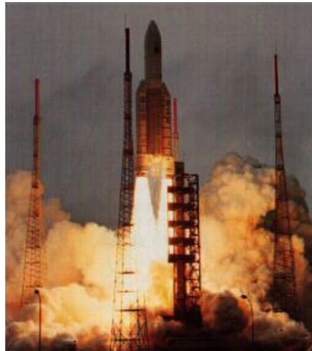
Illustration 3: An Ariane-5 rocket self-destructed after takeoff due to software error caused by an incorrect type conversion. The cost of this mistake was over 370 million dollars. Photo: ARIANE 5 Flight 501 Failure Report by the Inquiry Board
