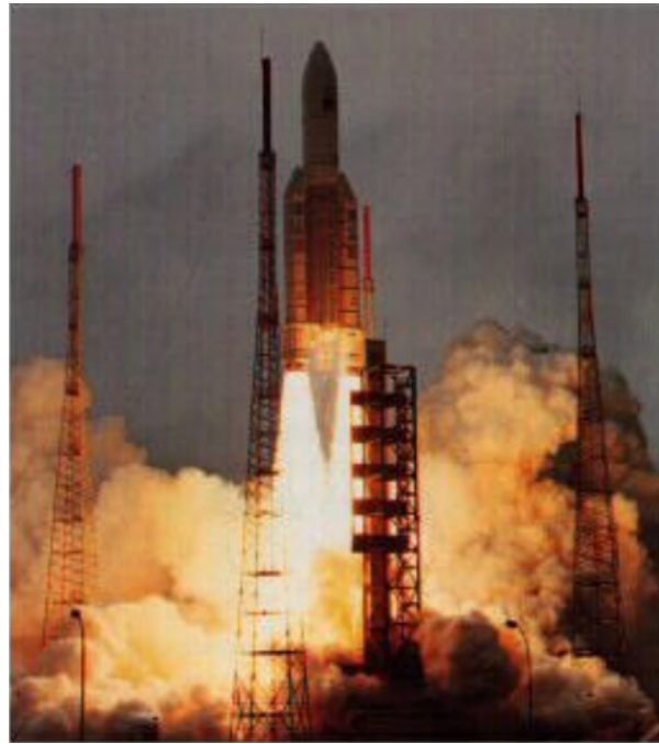
Figure 2.13: An Ariane-5 rocket self-destructed after takeoff due to software error caused by an incorrect type conversion. The cost of this mistake was over 370 million dollars. Photo: ARIANE 5 Flight 501 Failure Report by the Inquiry Board ( http://sunnyday.mit.edu/nasa-class/Ariane5-report.html ), Public Domain
