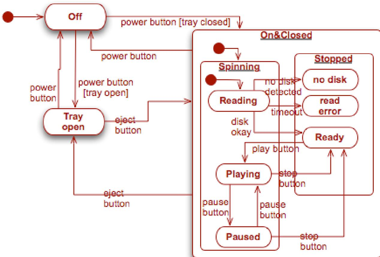
Note: this model assumes that the player can be off with the tray open. In fact most DVD players automatically close the tray before turning off. This can be modeled by adding "close" as an action to the transition from "Tray open".
