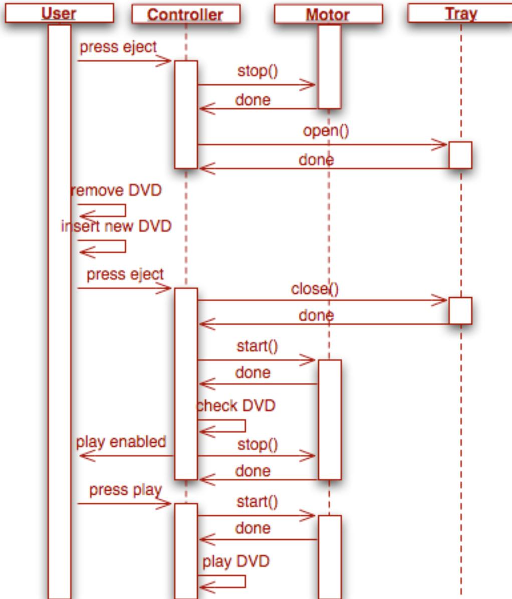
This answer assumes that the DVD player is unable to detect the actions of removing and inserting a disk while the tray is open, hence these actions are only relevant to the user. It also assumes that the controller is responsible for reading the disk once the motor is spinning, and will enable the play buttons at the same time as it turns off the motor, once it has successfully checked the disk.
