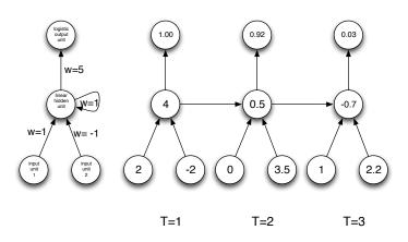
Assume we have a sequence of binary inputs. We'll consider how to determine the parity, i.e. whether the number of 1's is even or odd.
