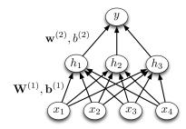
All of the hidden units and the output unit use a hard threshold activation function:
