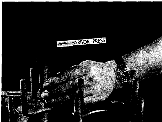
Figure 118 — Installing valve seat insert with an arbor press
