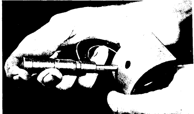
Figure 143 — Measuring Bearing Thickness
