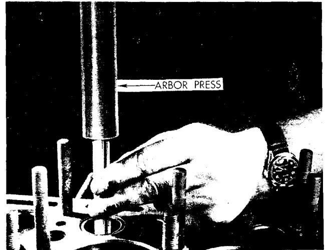
Figure 115 — Removing valve guides
