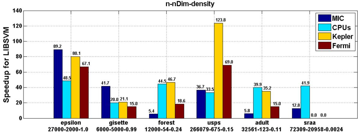
Fig. 11. This figure shows the speedups over LIBSVM based on the time of each iteration (rather than the whole time),  $n$  is the number of training samples,  $nDim$  is the dimension of each training sample, and density represents the sparseness of a given dataset. All the results data shown in this figure are the average of many runs.
