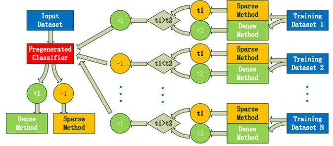
Fig. 4. The figure shows our adaptive support for different types of datasets in our MIC-SVM. The pre-generated classifier is trained through  $N$  ( $N \geq 100$ ) different real-world datasets which cover a variety of patterns.
