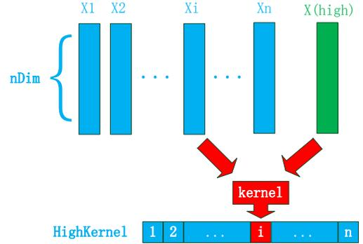
Fig. 3. This figure corresponds to the computation of  $HighKernel$  (used in Equation (11)).  $HighKernel$  is a vector, and  $HighKernel(i) = \text{Kernel}(X_{high}, X_i)$ . From this figure we can see that the evaluation of  $HighKernel$  need to access all the training samples. The computation of  $LowKernel$  can be accomplished in the same way.
