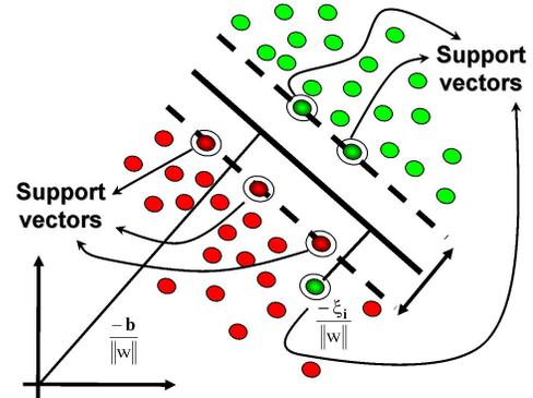
Fig. 1. The figure shows Support Vector Machines, whose decision boundary is decided by Support Vectors (SVs). The left-lower dots represent the -1 class and the right-upper dots represent +1 class. These two classes are classified by the the decision boundary (the dashed lines in this figure). We can observe that the classification result is decided by the six Support Vectors.
