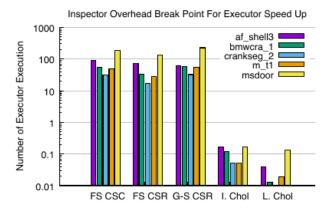
**Figure 10.** This figure shows how many times we need to run the executor for a benchmark given a specific input matrix in order to cover the inspector overhead and gain speedup. The X-Axis shows cluster of bars for each benchmark code, each bar being the number of needed run for a specific input matrix. The numbers in the Y-axis are  $(inspector_t + executor_t)/(serial_t - executor_t)$ . Please note Y-axis is in log scale.
