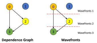
**Figure 2.** Dependence graph for forward solve for sparse matrix in Figure 1.
