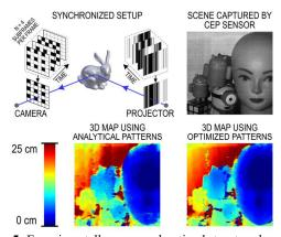
**Fig. 5:** Experimentally measured optimal structured-light 3D imaging results.
