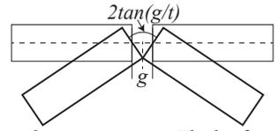
The maximum curvature of the bend, number of cuts, kerf width and material thickness are all linked by simple geometric formulas, as seen inset.
