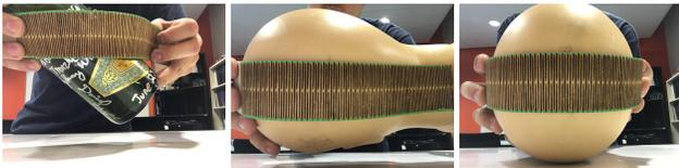
**Figure 5: Images of Bend-a-rule wrapped around 3D objects.**
