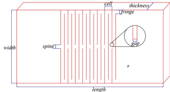
Figure 9: Bend-a-rule construction parameters.
