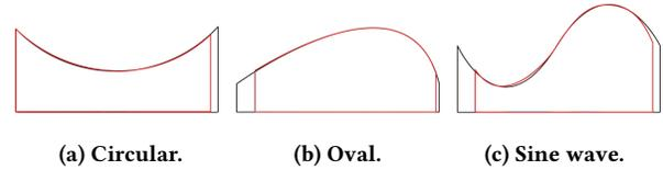
Figure 8: Curves acquired using Bend-a-rule (red) are shown superposed over example ground truth curves (black).
