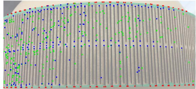
**Figure 6: Corner detection methods:** ours (red), Harris (green), and SURF features (blue).
