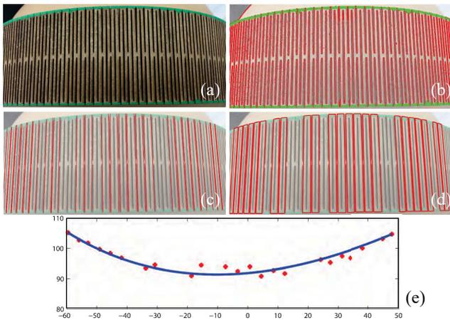
**Figure 4: Reconstruction Algorithm:** the original image (a), is processed to extract boundary curves as green pixels using mean-shift clustering and lattice cell edges as red pixels using image gradients (b); lattice edges are refined by RANSAC (c), and intersected with the boundary curves to define lattice cells (d). 2D projections of the homography reconstructed cell centers and a best-fit smooth curve (e).
