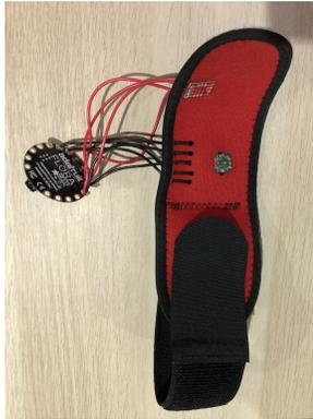
access to raw sensor data at sub-second granularity (Apple). Readings are collected and synchronized from sensors using a microcontroller at a rate of 25Hz.
