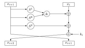
Fig. 4: One Fiestel round of Simon cipher. Diagram from [36].
