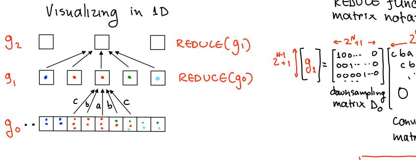
REDUCE function in matrix notation (1D) convolution matrix Co
