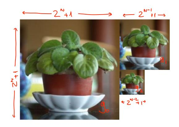
The elements of a Gaussian Pyramids are smoothed copies of the image at different scales.
