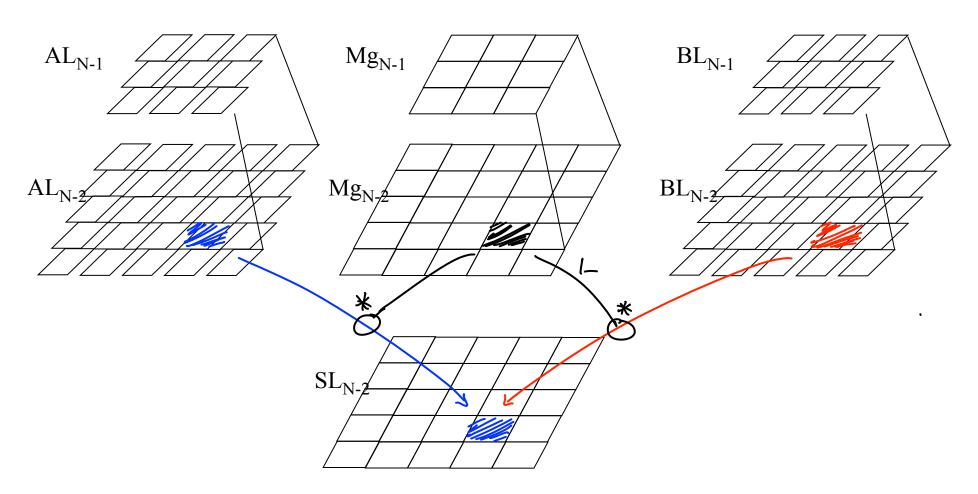
(4) Compute the Laplacian pyramid, SLo, SL1,...SLin-1, Sgn by applying the matting equation with matter Mge: SLe(i,j) = Mge(i,j) ALe(i,j) + (1-Mge(i,j)) BLe(i,j)
