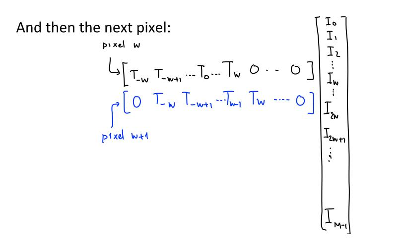
Then, the cross correlation at pixel w can be computed using:
