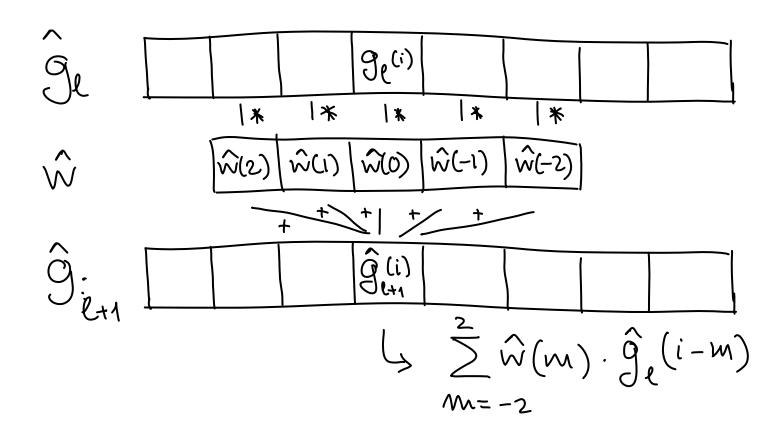
This means that to estimate the i<sup>th</sup> pixel at the (l+1)<sup>th</sup> level one must do:
