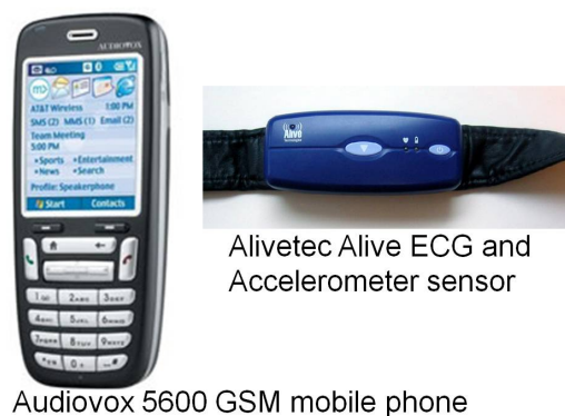
Figure 3. TripleBeat's Hardware. Left: Audiovox SMT5600 mobile phone. Right: Alivetec Alive heart monitor.
