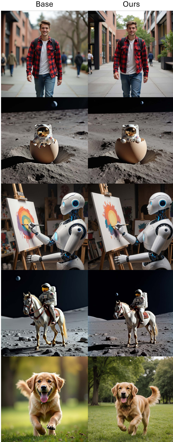
Fig. 2. Qualitative comparison between the baseline FLUX model and our training-free focus-control method. Our approach produces noticeably sharper background regions while preserving subject clarity, demonstrating improved depth-of-field control across diverse scenes.
