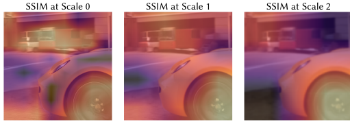
Fig. 4. Difference heatmaps across spatial scales for the low-level SSIM metric. Notice that highlighted regions are generally blob-like, and subtle visual differences (e.g., car wheel) are detected.
