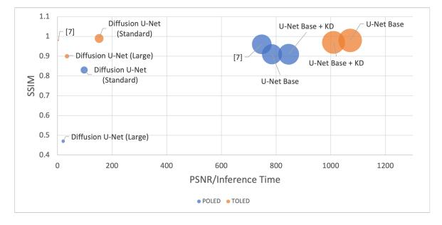
Fig. 5. SSIM vs. PSNR/Inference Time for various approaches. Scale of each circle is the product of its values on each axis.
