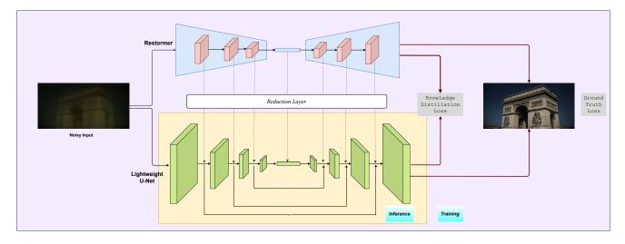
Fig. 2. The teacher model is Restormer [4] which is pre-trained and frozen, the lighter student model is a U-Net that does 4x downsampling and upsampling.
