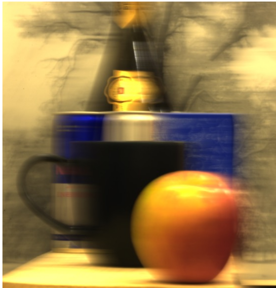
parabolic input - blur is invariant to velocity
