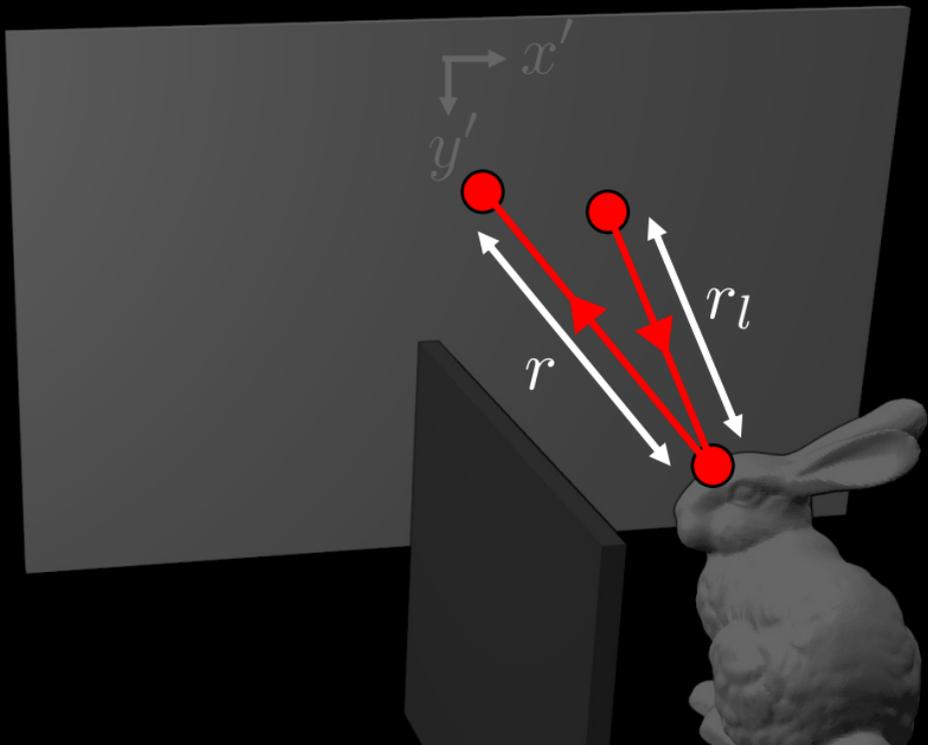
$$\tau(x', y', t) = \iiint_{\Omega} \underbrace{\frac{1}{r_l^2 r^2}}_{\text{radiometric term}} \underbrace{\delta(r_l + r - tc)}_{\text{geometric term}} \cdot \underbrace{\rho(x, y, z)}_{\text{hidden 3D volume}} dx dy dz$$
