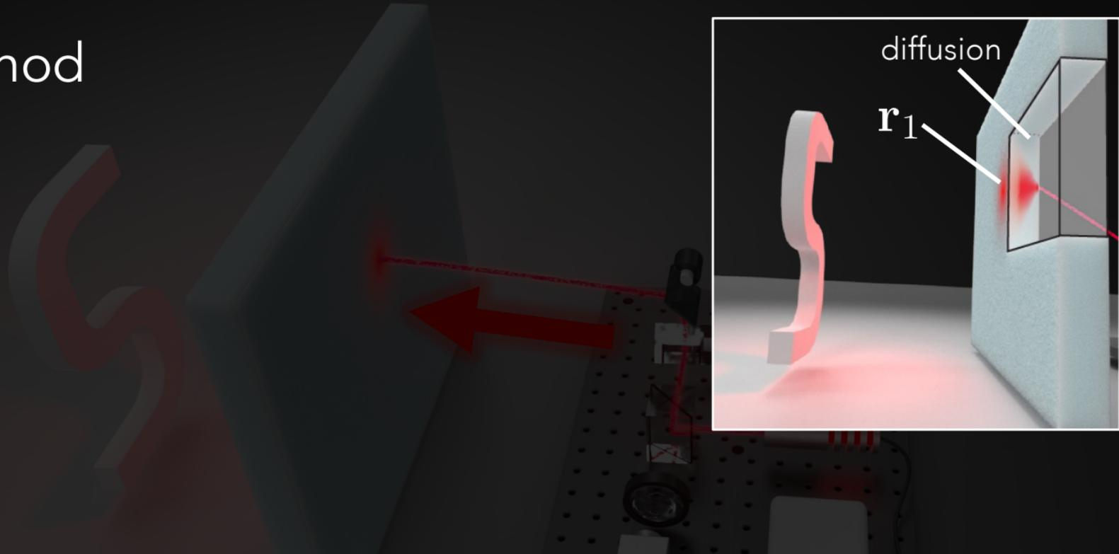
$$\phi(t, \mathbf{r}_0, \mathbf{r}_1) = \frac{c}{(4\pi Dct)^{3/2}} \exp\left(-\frac{\|\mathbf{r}_1 - \mathbf{r}_0\|_2^2}{4Dct} - \mu_a ct\right)$$
