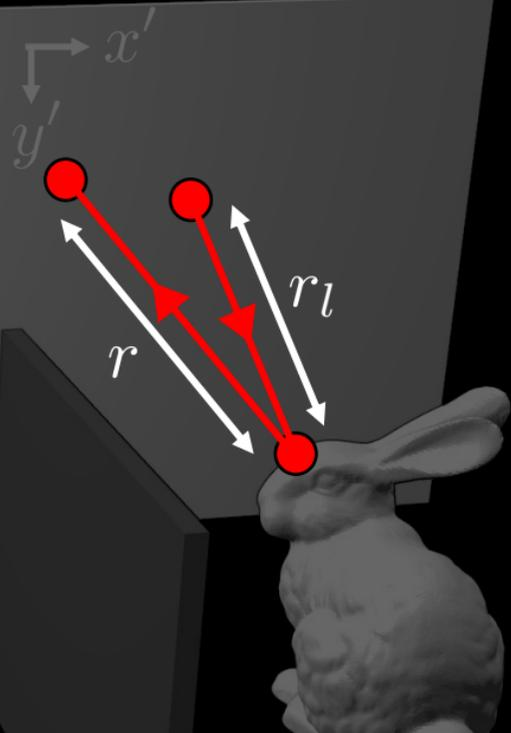
$$\tau(x', y', t) = \iiint_{\Omega} \frac{1}{r_l^2 r^2} \delta(r_l + r - tc) \cdot \rho(x, y, z) dx dy dz$$
