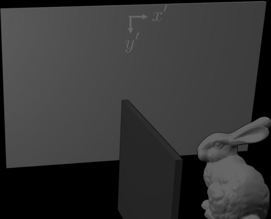
$$\underbrace{\tau(x', y', t)}_{\text{3D measurements}} = \iiint_{\Omega} \underbrace{\frac{1}{r_l^2 r^2}}_{\text{radiometric term}} \underbrace{\delta(r_l + r - tc)}_{\text{geometric term}} \cdot \underbrace{\rho(x, y, z)}_{\text{hidden 3D volume}} dx dy dz$$
