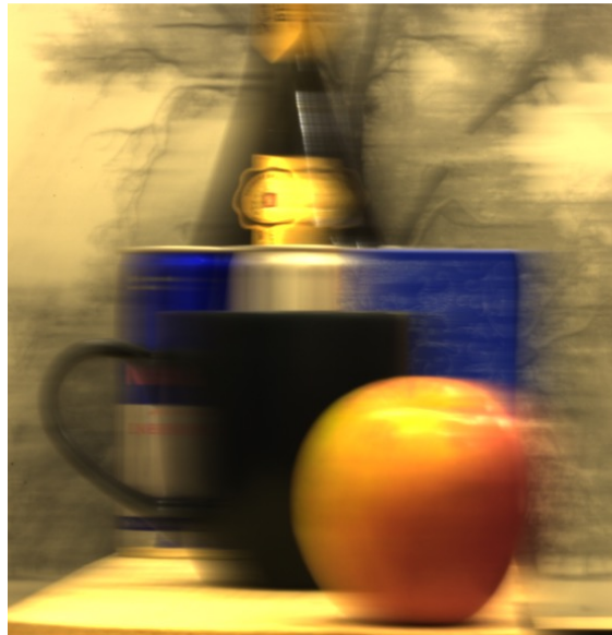
parabolic input - blur is invariant to velocity
