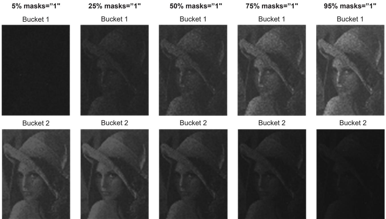
Figure 7. Capturing a photo of Lena shown on the computer screen, while changing the level of pixel masking. The number of masks equal to one starts from 5% on the left, and increases all the way up to 95% on the right. The output image is shown for each of the buckets.
