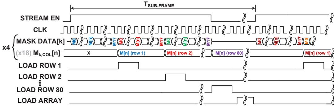
Figure 4. A simplified waveform diagram of the mask deserialization and loading.
