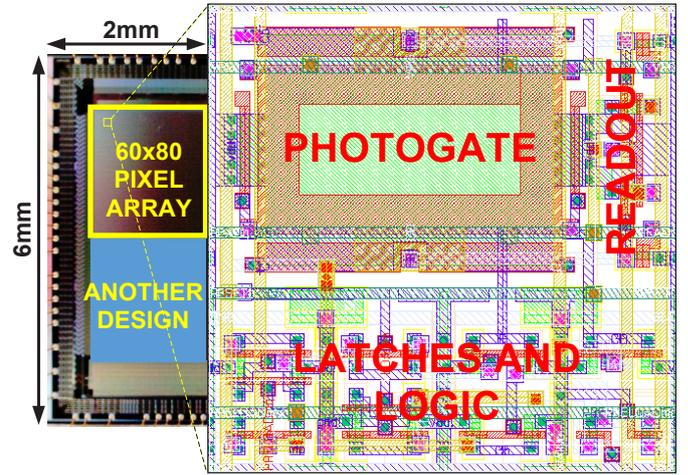
Figure 6. The pixel layout and the image sensor die micrograph showing the chip region dedicated to PDC.
