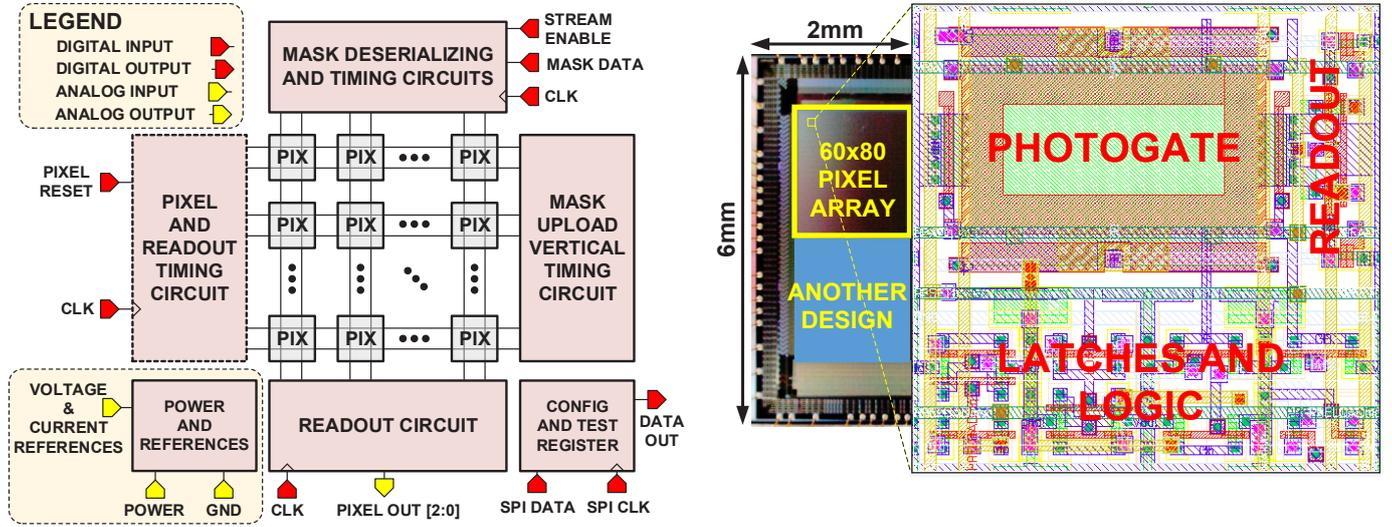
Figure 5. The proposed PDC CMOS image sensor architecture.
