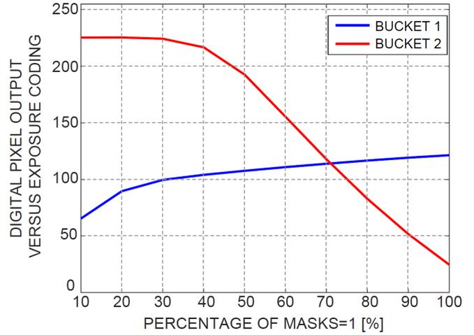
Figure 3. The measured digital pixel output at uniform light versus the coded pixel exposure expressed as percentage of masks applied over the complete frame exposure.
