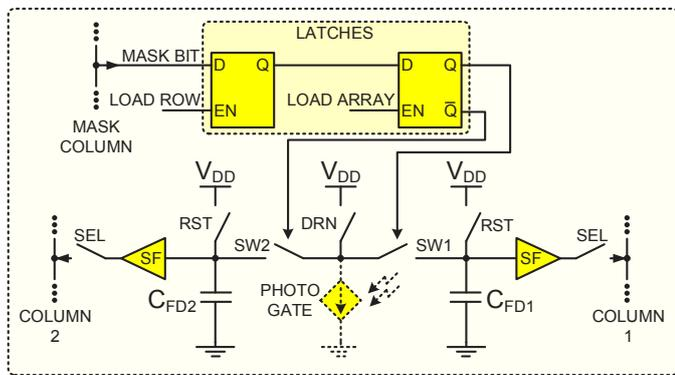
Figure 2. The proposed PDC pixel circuit diagram with level-sensitive latches.
