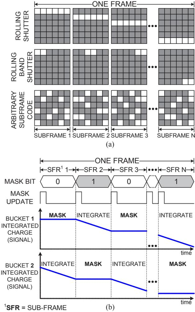
Figure 1. An illustration of the electrical coded-exposure implementation: (a) coded-exposure imaging examples of the typical PDC masks that could be applied over many different subframes, (b) pixel timing diagram of the related pixel signal integration process depending on the masking bit value over multiple subframes.
