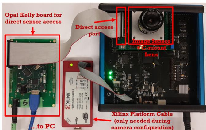
Figure 8. The complete sensing side of the imaging system with the camera system and the FPGA board used for the direct signal acquisition.
