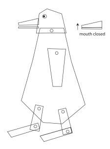
It has six rotational joints (depicted by circles), each with one rotational degree of freedom. The beak has a single translational degree of freedom: the beak can only move up or down (in the coordinate frame of the head). Your task will be to render and animate such a robot penguin using OpenGL.
