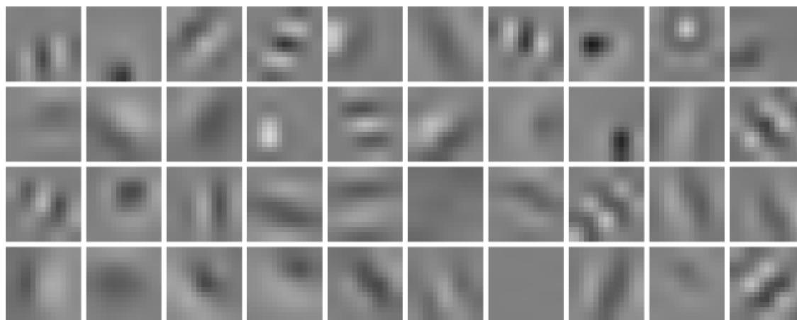
Fig. 2 Examples of the first layer filters learned by our deep convolutional neural net. These filters have resemblances to human-designed feature extractors such as edge, spatial-frequency, texture and interest point detectors from computer vision.
