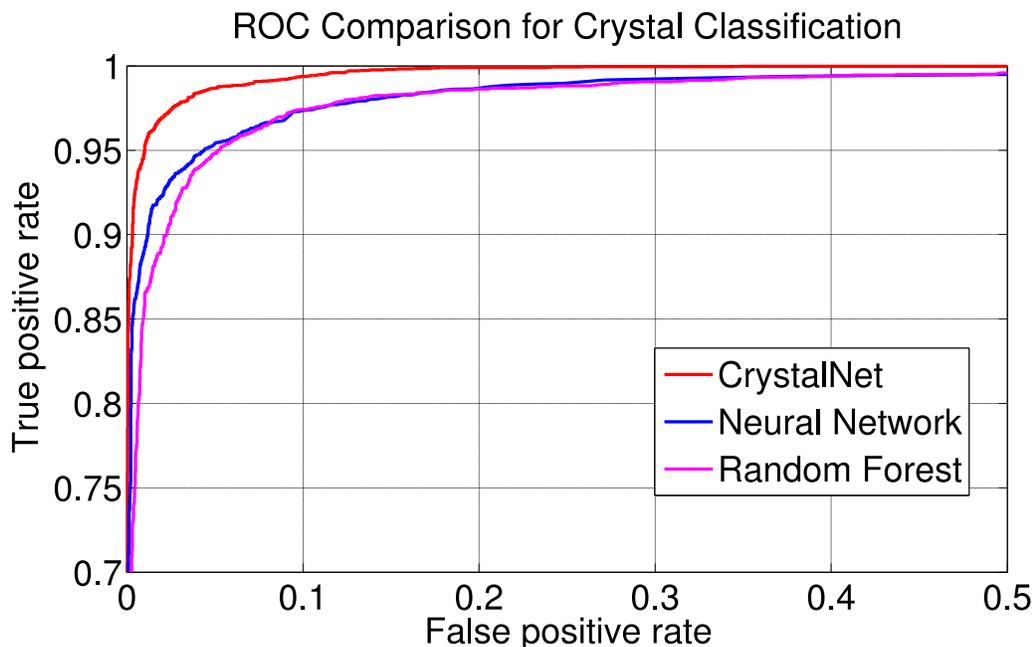
Fig. 3 ROC curve for bi-classification of crystal
