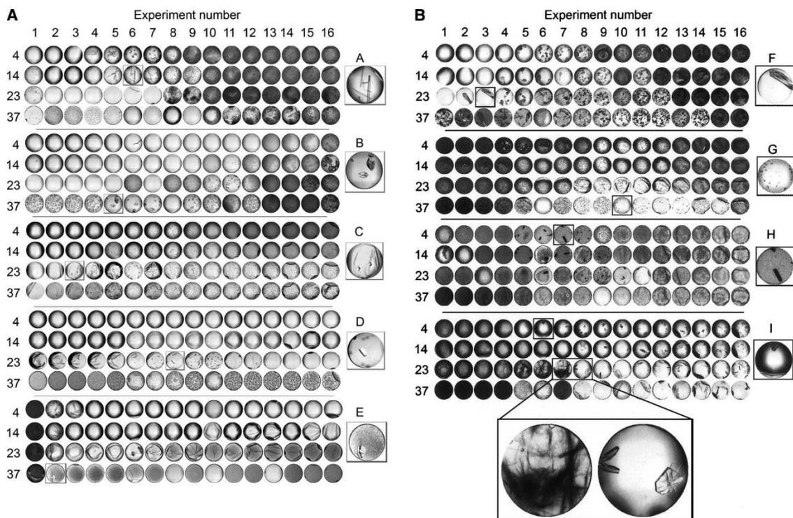
Figure 1: Protein crystal optimization using Hauptman-Woodward's Drop-Volume Ratio/Temperature method. Nine different optimization matrices are shown. The protein/cocktail ratios are highest for column 1 and lowest for column 16. Temperatures in centigrade are marked in the rows. Source: Luft, J. R., Wolfley, J. R., Said, M. I., Nagel, R. M.,
