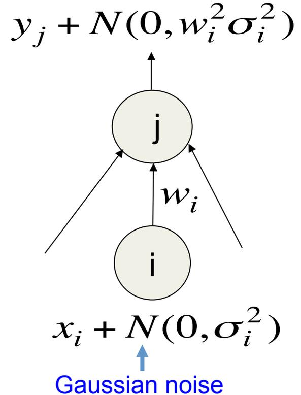
output on one case  $\rightarrow y^{noisy} = \sum_i w_i x_i + \sum_i w_i \varepsilon_i$  where  $\varepsilon_i$  is sampled from  $N(0, \sigma_i^2)$
