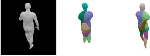
Figure 5: Comparison between Free Cerberus (w/o pose consistency) and Cerberus (w/ pose consistency). **Left:** Input. **Middle:** Output of Free Cerberus. **Right:** Output of Cerberus. Free Cerberus uses a single green part for 2 legs while Cerberus correctly models 2 legs.
