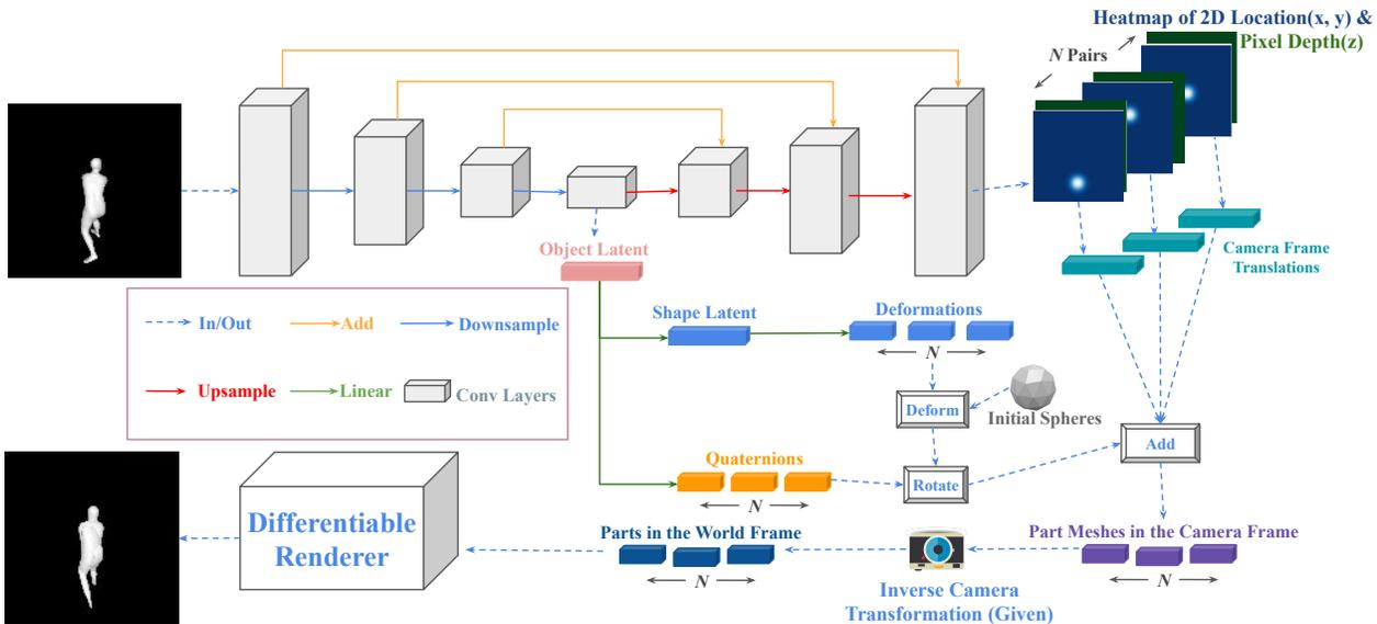
Figure 2: Cerberus architecture. Here we visualize 3 out of  $N$  parts used in the pipeline. Up-sampling is performed by de-convolution. The object latent is obtained by global average pooling of the lowest-resolution feature maps. Predicted quaternions are used to construct rotation matrices.
