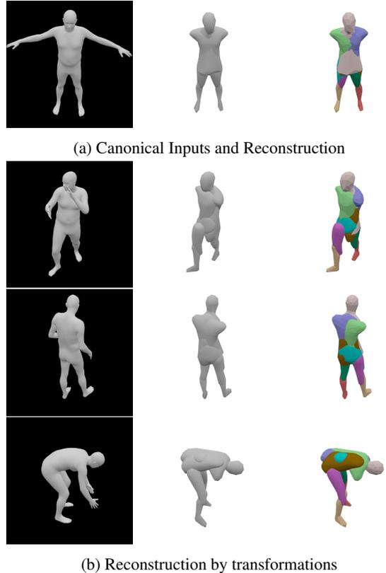
Figure 4: Hard human reconstruction test. We extract a single set of deformed shape meshes from the canonical inputs (a) and apply new transformations (rotation and translation) predicted from other images to these meshes to reconstruct new poses (b). **Left:** Input images. **Middle:** Reconstructed 3D outputs. **Right:** Parts rendered in different colors.
