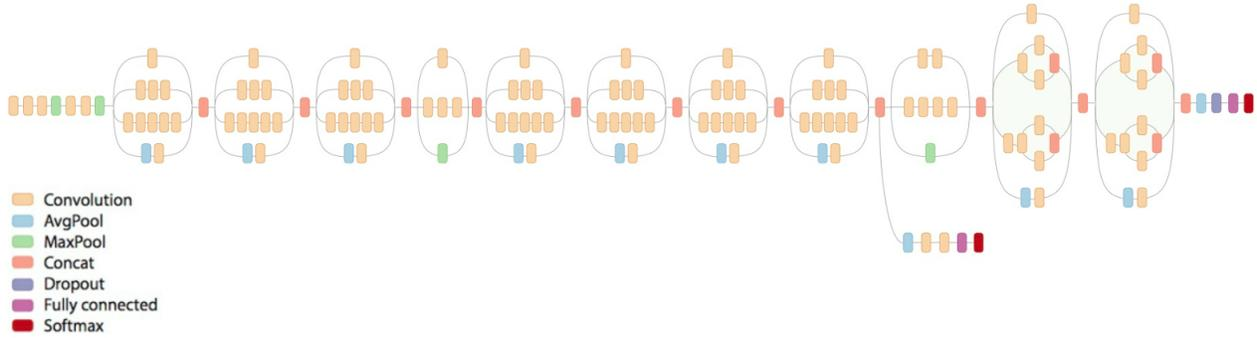
Figure 6: Schematic diagram of Inception-v3 (Shlens 2016).
