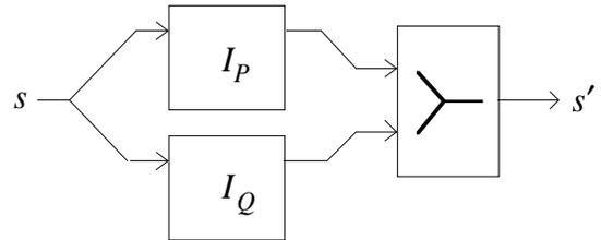
This implementation of parallel composition allows  $P$  and  $Q$  to access memory simultaneously. For the memory we have described, simultaneous access to different variables or arrays poses no problem. Even for the same variable, simultaneous reads are no problem. But simultaneously reading and writing the same variable, or two simultaneous writes to the same variable, have unpredictable results. We
