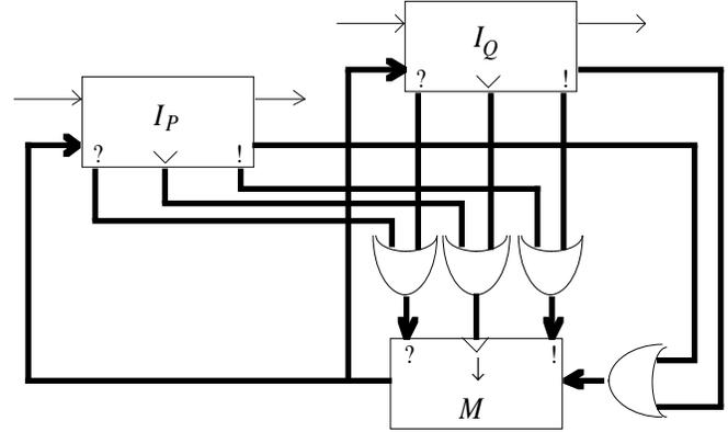
Each disjunction is really many disjunctions, one for each bit in its operands.
