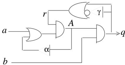
Internal wires can be left exposed, as in the above specification of 1-2-merge and the top diagram, or they can be hidden as in the bottom diagram and the following specification:
