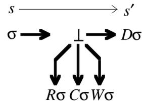
We have shown all its inputs and outputs. But since the  $\sigma$  input is not connected to anything, there is no point in bringing those wires from memory. And since the  $R\sigma$ ,  $C\sigma$ ,  $W\sigma$ , and  $D\sigma$  outputs are  $\perp$ , there is no point in taking them into a disjunction. So the circuit reduces to nothing, which is appropriate for a circuit that does nothing.
