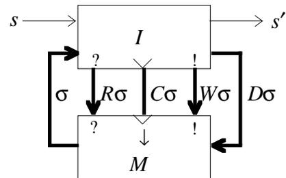
A thin line indicates one wire; a thick line indicates many wires. We are depicting logic, not layout; the best place for a bit of memory may be with a part of the control that uses
