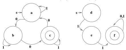
The machine on the left is  $M_1$ , and the one on the right is  $M_2$ .
