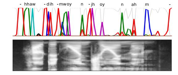
CTC does not require prior segmentation because the network is free to emit the labels at any time, as long as their order is correct. It also allows the labellings to be read straight from the network outputs (follow the spikes).
