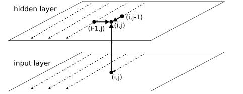
This gives the network access to multidimensional context, and makes it robust to local distortions that 'mix' dimensions, such as shears, rotations etc. To get context from all directions, we scan through each n-dimensional data sequence with  $2^n$  separate networks, starting in every corner.
