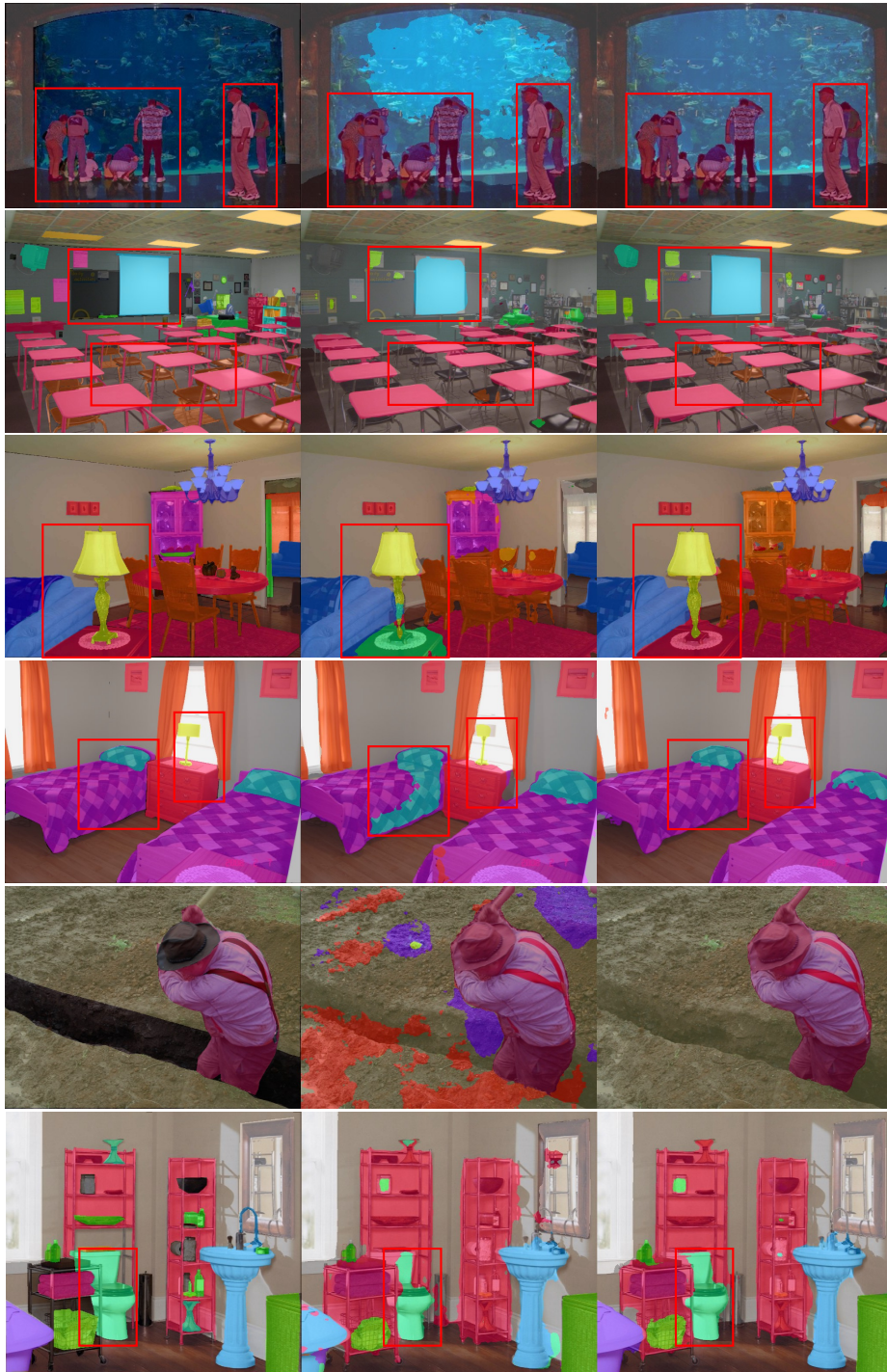
Fig. 14: Qualitative comparisons on ADE20K. We compare our method with the SegFormer baseline and highlight the differences using red rectangles. Our predictions conform to boundaries object boundaries much better, and in some cases, surpasses the coarse ground truth masks.
