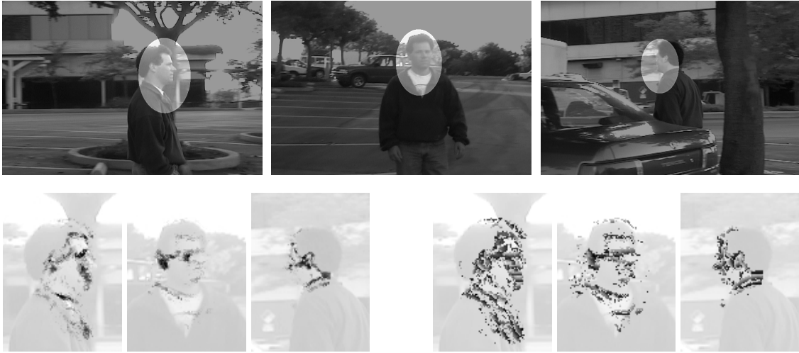
Figure 4. The adaptation of the model during tracking. (top) The target region in selected frames 200, 300, 480. (bottom) The stable component’s mixing probability (left) and mean (right) for the selected frames.
