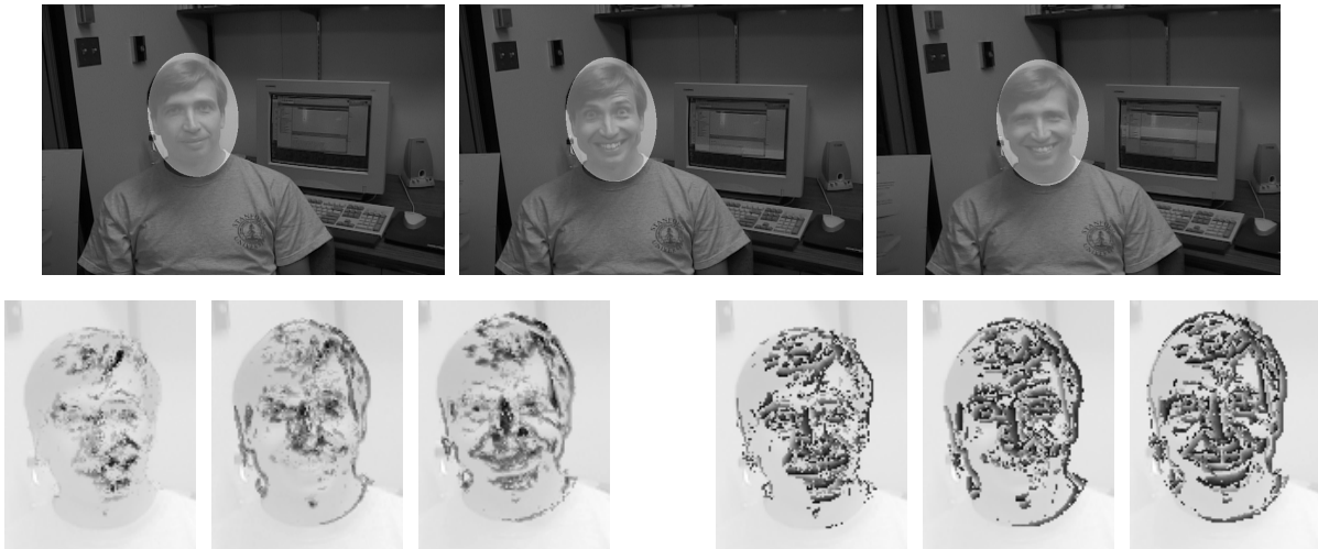
Figure 5. Adaptation to changes of expression. (top) The target region in selected frames 420, 455, 490. (bottom) The stable component’s mixing probability (left) and mean (right) for the selected frames (time increases left to right in each set). Note how the regions around the mouth and eyebrows adapt, while others remain stable.
