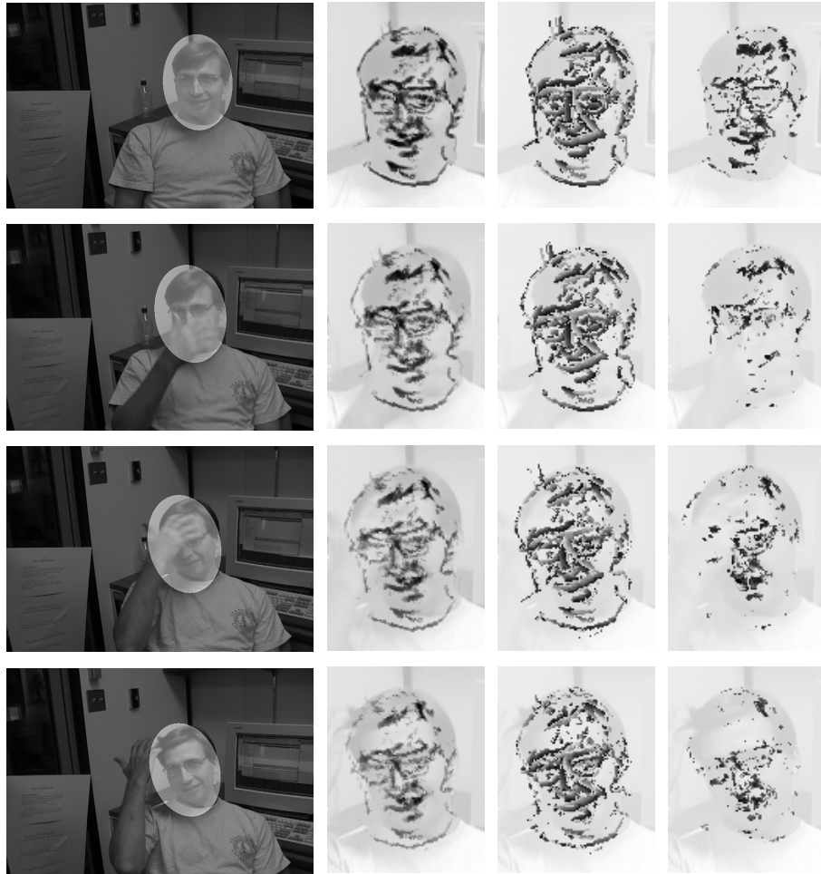
Figure 6. Robust tracking despite occlusion. Tracking results for frames 200, 205, 210 and 215 are shown, top to bottom. The elliptical tracking region, and the stable model’s mixing probability, mean and ownership are arranged left to right. Note that the model is misaligned during the occlusion (see the second and third images on the second row) but that it promptly realigns. Also, note the stability and model persistence (left three columns), along with the reduced data ownership on the hand (right column).
