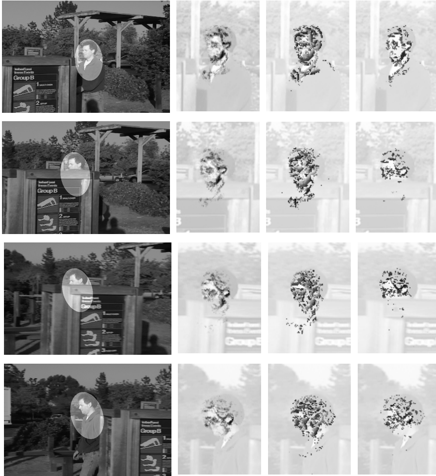
Figure 3. Each row shows, from left to right, the tracking region, the stable component’s mixing probability m_s(\mathbf{x}, t) , mean \mu_s(\mathbf{x}, t) , and ownership probability o_s(\mathbf{x}, t) . The rows correspond to frames 244, 259, 274, and 289, top to bottom. Note the model persistence and the drop in data ownership within the occluded region.
