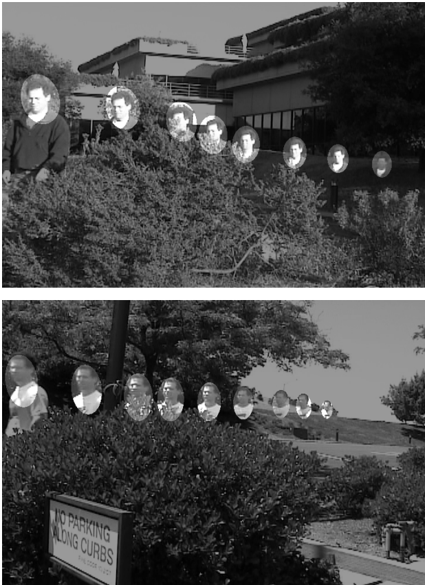
Figure 7. Tracking with partial occlusion along with variable lighting, appearance and size. The camera was stationary, and the sequences are each roughly 250 frames. We show the highlighted target region for selected frames superimposed on the last frame.
