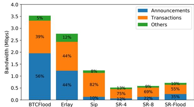
**Figure 7: Bandwidth consumption breakdown at 500 TPS workload throughput and 20Mbps bandwidth limit.**
