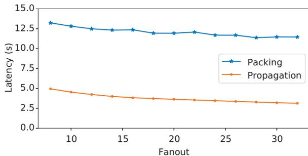
**Figure 11: The average transaction propagation and packing latency of different fanouts.**
