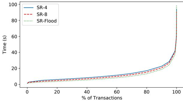
**Figure 10: Transaction packing latency with 20 Mbps bandwidth limit.**
