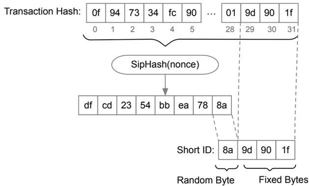
Figure 1: Transaction short id encoding in Shrec.
