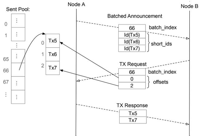
Figure 3: The normal flow of node interaction in Shrec.
