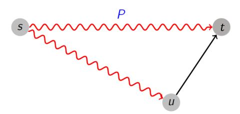
• OPT(t, i) = length of the shortest path from s to t using at most i edges
