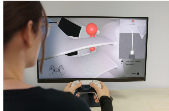
Fig. 1: User controlling the continuum robot simulator with a gamepad controller. The screen displays the user interface, including two views of the application task.
