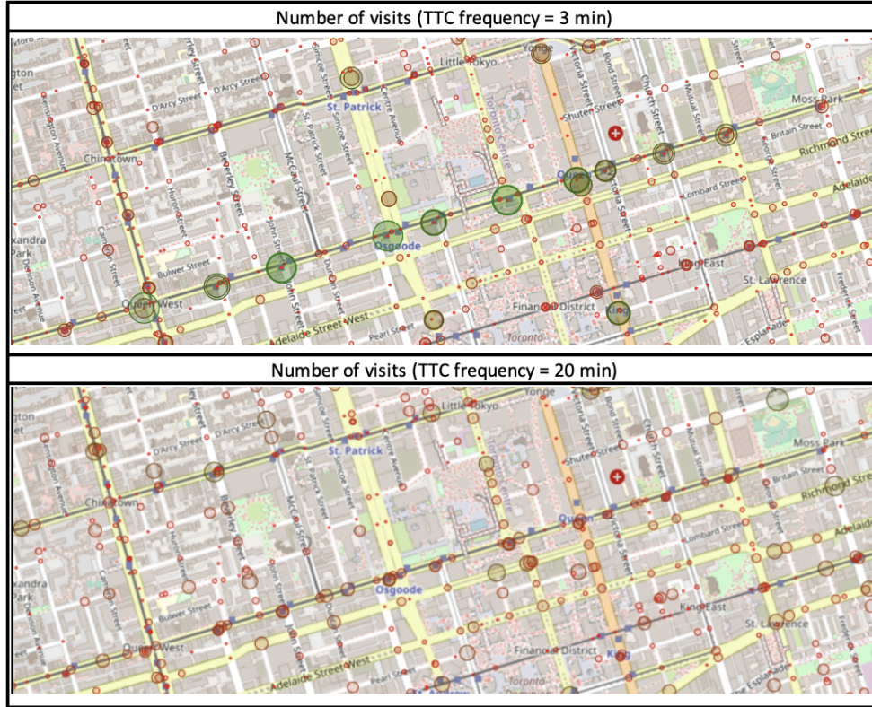
Figure 19: Individual nodes visits depending on TTC frequency on a small fragment of the map
