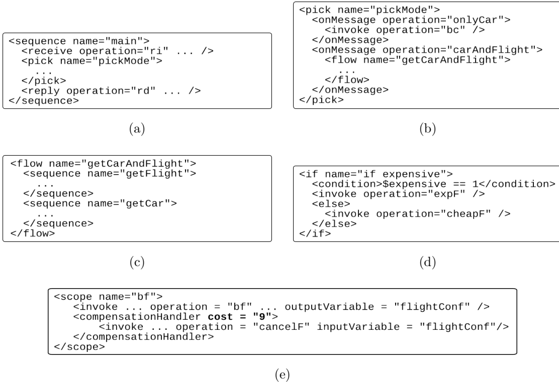
Figure 2.5: BPEL specification of selected TAS activities: (a) the main process; (b) <pick> labelled ①; (c) <flow> labelled ②; (d) <if> labelled ③; and (e) compensation for booking a flight (bf).
