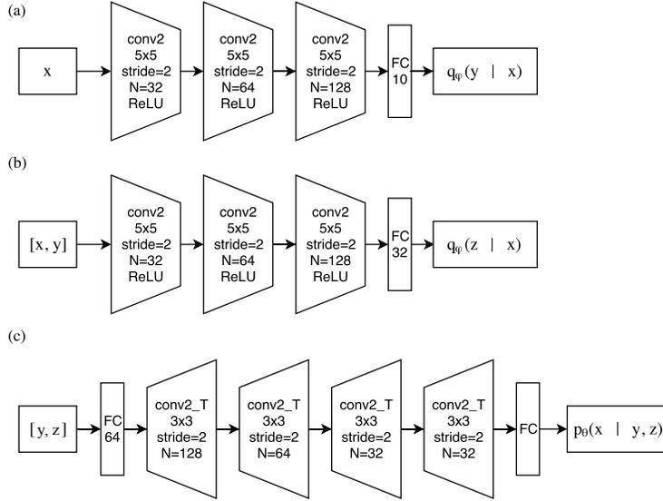
Figure 7: Network architecture for (a) classification  $q_\phi(y|x)$  (b) inference  $q_\phi(z|x, y)$ , and (c) generative  $p_\theta(x|y, z)$  models. The output of these networks parameterize Categorical, Gaussian, and Bernoulli distributions which we sample from.
