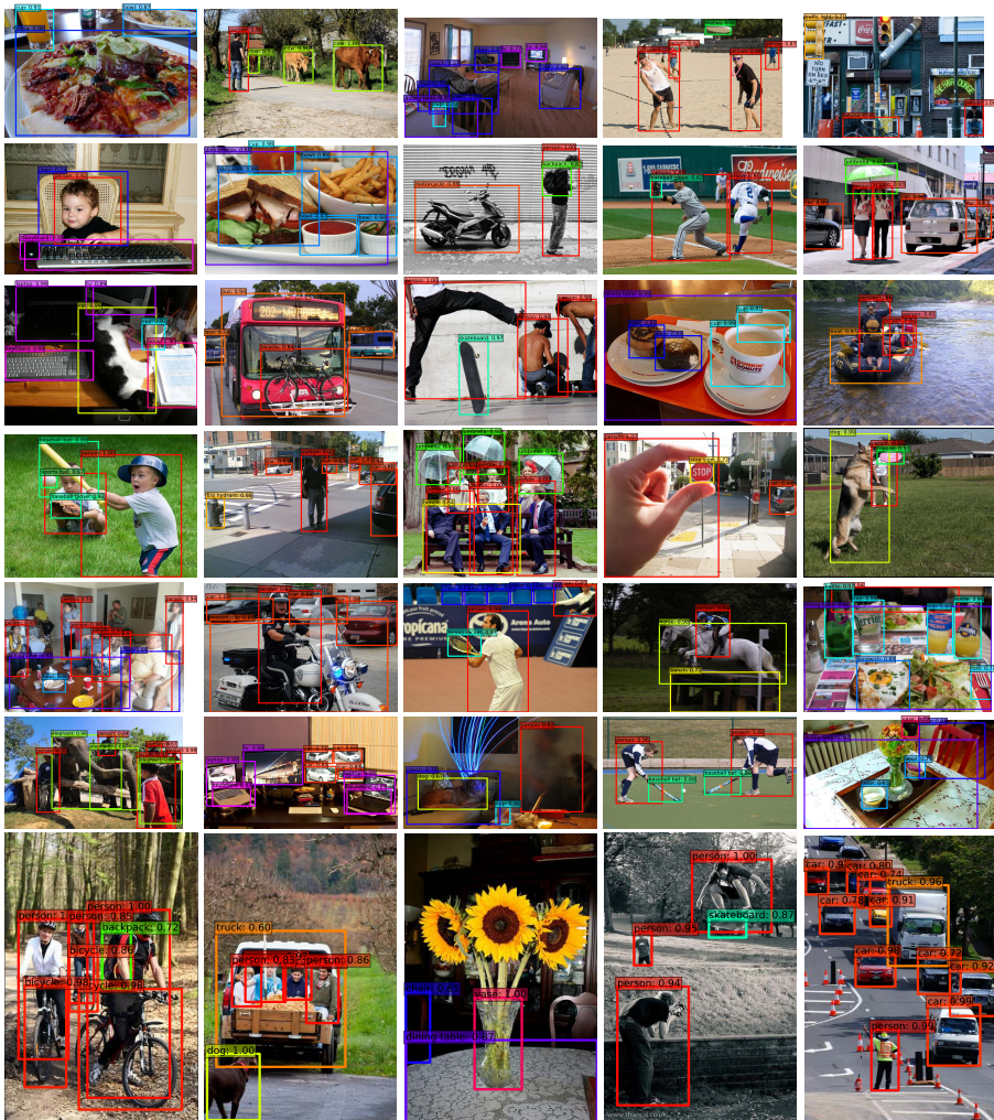
Fig. 5: Detection examples on COCO test-dev with SSD512 model. We show detections with scores higher than 0.6. Each color corresponds to an object category.
