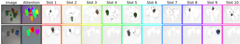
Figure 6: Visualization of the attention masks on CLEVR10 for two examples with 9 and 4 objects, respectively, for a model trained on the property prediction task. The masks are upsampled to 128 \times 128 for this visualization to match the resolution of input image.
