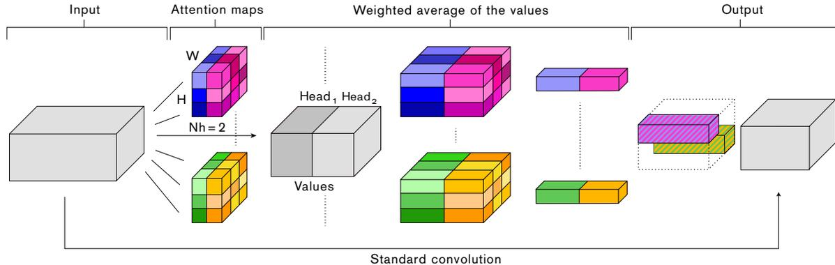
Figure 2. **Attention-augmented convolution**: For each spatial location  $(h, w)$ ,  $N_h$  attention maps over the image are computed from queries and keys. These attention maps are used to compute  $N_h$  weighted averages of the values  $V$ . The results are then concatenated, reshaped to match the original volume’s spatial dimensions and mixed with a pointwise convolution. Multi-head attention is applied in parallel to a standard convolution operation and the outputs are concatenated.
