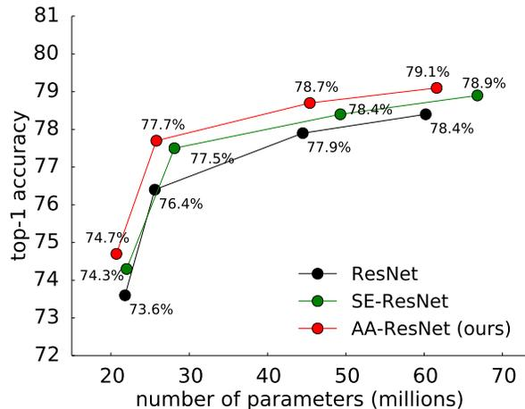
Figure 1. **Attention Augmentation systematically improves image classification across a large variety of networks of different scales.** ImageNet classification accuracy [9] versus the number of parameters for baseline models (ResNet) [14], models augmented with channel-wise attention (SE-ResNet) [17] and our proposed architecture (AA-ResNet).
