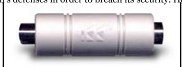
Cybercrime no longer requires exceptional technical skills. This perfectly innocuous device is actually a hardware keyboard logger which silently and undetectably captures key strokes! They can be bought online for less then $100 US.
